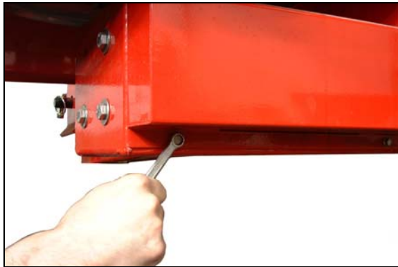
1. Loosen screws securing the lower guard.
