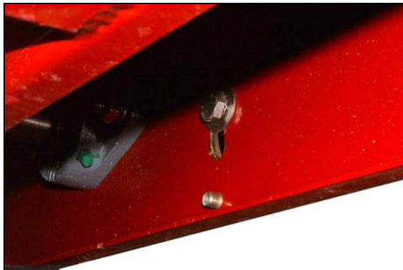
3. Loosen screw securing the belt-tensioner.
