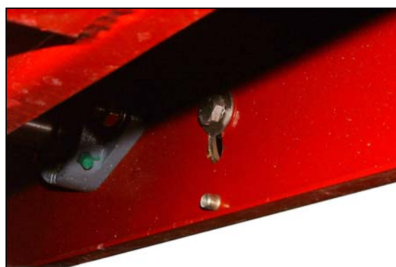
5. Tighten screw securing the belt-tensioner.
